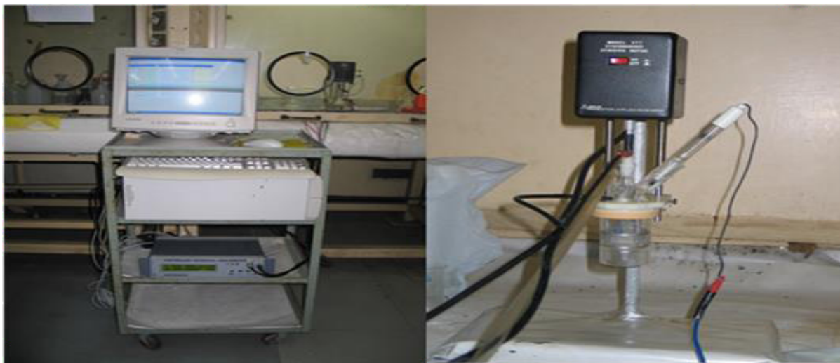
Figure 3. Coulometric setup employed for quantification of U and Pu in nuclear fuel samples.
